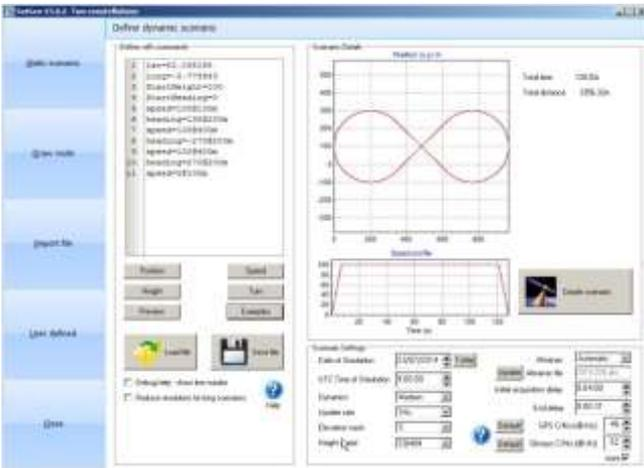
A suitable almanac can be automatically downloaded, or defined by the user. **SatGen** can also import KML files and NMEA files, and the time, date and dynamics are fully user definable.
